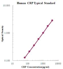
A standard curve must be run within each assay. The following standard curve is provided for demonstration only.
